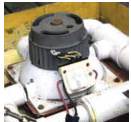
The four-nozzle Harris turbine generates 3.6 KWH per day.
