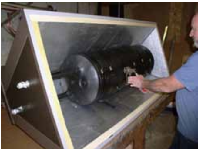
Adding glass and trim will complete the batch heater.
