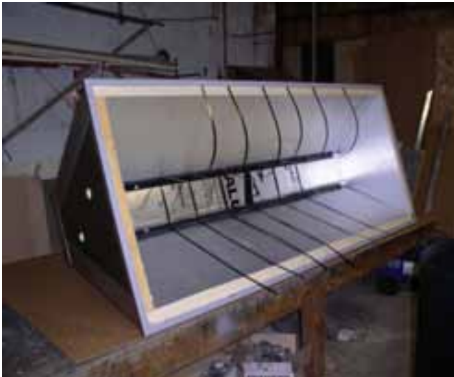
Steel strapping holds the tank in the batch heater.
